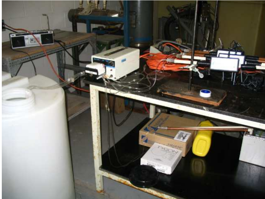
Photo 2: Water line synthetic water supply systems
