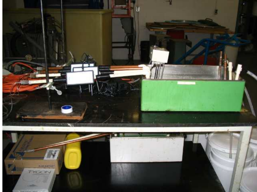
Photo 1: Scalehammer installed on the water lines
